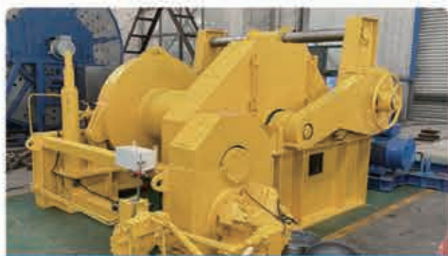
Multi-point mooring and positioning winches
