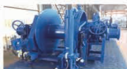
Tractor Winch Anchor Removal Winch
